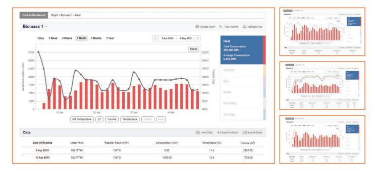
With a remote monitoring system you can access a data visualisation tool that will give you complete visibility and control of your biomass system 24/7 and in real time. The user-friendly, online dashboard allows you to analyse the kWh generation and usage data for each heat meter and view the Herz boiler T-Control interface. What's more, the tool is cloud based so it is extremely fast and can be accessed via a smartphone, tablet or PC.
