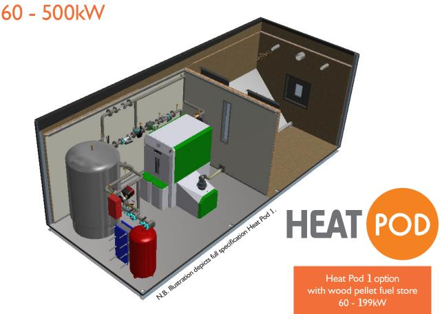
Heat Pods are an all-in-one pod consisting of a Herz biomass boiler, plant room, pipework and a fuel store. This range has two models depending on the size of biomass boiler required.
